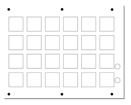
Once your graphic overlay is printed you will need to use a hole punch make the holes in the graphic overlay in the locations shown on the PDF design template, so that the graphic overlay will line up with the membrane buttons on the Digital Listening Station. Then open up the hinged panel as pictured below and insert your graphic overlay.
