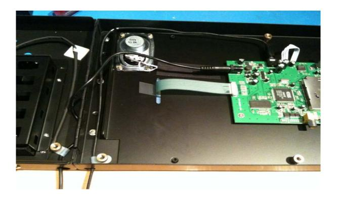
If you would like to disconnect the built-in stereo speakers, so that you can only hear audio from the headphones, disconnect the speaker wire from the circuit board by pulling out the plastic connector that is attached to white speaker wire as shown below.
