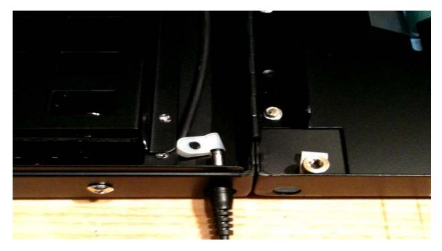
Remove the gold nut from the screw post and as shown and open up the plastic clamp. This will allow you to feed the power cord through the hole and the plastic clamp and plug the cord into the same port that you removed the battery cable from. At the top of the next page you will see a picture of what this should look like once installed.
