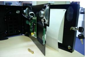
To power your Digital Listening Station you can use either 8 qty D-Cell Alkaline Batteries (not included) or the standard US Power Supply (included). The unit comes with the battery lead plugged into the board. If you would like to set up the unit to have temporary battery power, simply remove the 4 screws that hold the battery cover down and insert D-Cell Alkaline batteries.
